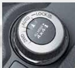
**Intuitive 4x4.** The ALL MODE 4x4-i system makes the Nissan X-TRAIL capable on-road and off. For maximum fuel efficiency choose 2WD. In Auto Mode conditions are constantly monitored and the balance of power between front and rear wheels is adjusted for best traction. Challenging conditions? 4WD Lock Mode is your choice.
