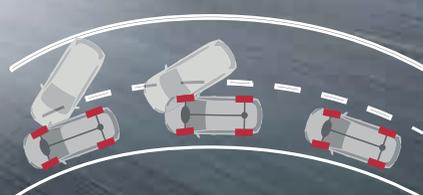
**Active Trace Control.** A turn for the better. This innovative technology helps improve control when you take a corner. It reads the cornering situation and, if needed, can brake each wheel individually to help you steer through the turn with confidence.
